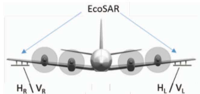
Figure 1 EcoSAR's dual antenna configuration. The antenna separation is 25m and both antennas are dual polarimetric capable of horizontal (H) and vertical (V) transmit and receive). Subscript R and L indicate right and left antennas.
