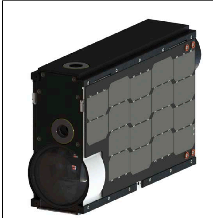
Figure 3-7 CAD View of 6U Spacecraft Stowed With 10 cm Telescope
