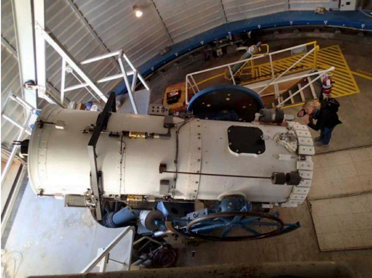
Figure 4-2: The 0.9 m SpaceWatch telescope from above. The dark rounded square plate would be the mounting plate for the demo telescope.
