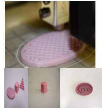
CRG FDM prints using reclaimed anti-static bagging film with reversible cross-linking additive
