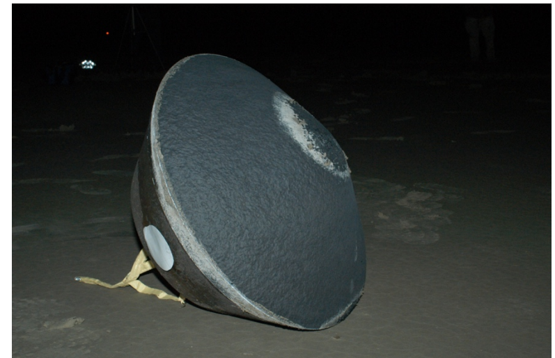
Stardust single piece, seamless heatshield
