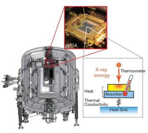
Low temperature ⇔ low heat capacity ∆E ~ 4-5 eV for 0.2-13 keV x-rays
