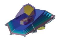
Origins Space Telescope (proposed) contains three instruments that require sub-Kelvin cooling. All three use TES detectors operating at 50 mK. At this temperature, the sensitivity will be limited by the sky background.
