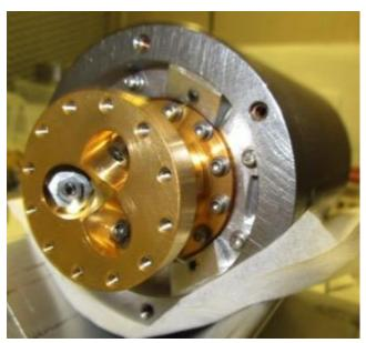
A total of 6 Kevlar bundles suspend the paramagnetic salt pill within the bore of a superconducting magnet
