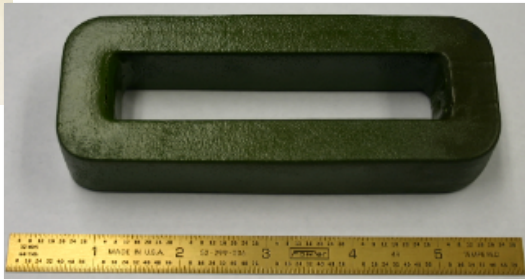
Transformer fabricated from spin cast ribbon
