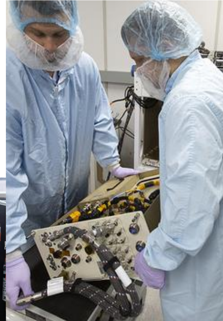
Power Distribution Assembly
