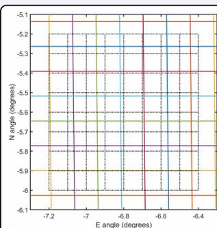
Figure 2: Conceptual illustration of GLM irregular angle resampler algorithm. Solid colored lines indicate the angular coordinates of the GLM pixels (lines are plotted every 10 pixels), and the regular "ABI-like" grid is shown in dotted black lines. A local search algorithm is employed to assign GLM pixel values to resampled pixels.
