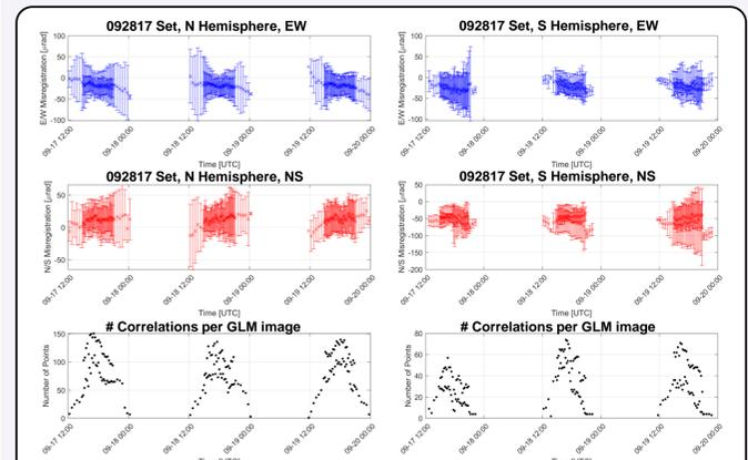
Figure 5: GLM NAV results for 3 days of GLM background images from September 2017. Quality filtering has been applied as described above. Results are shown as a function of GLM background image acquisition time, on a per-image basis. Error bars on the EW and NS plots are  $\pm 3\sigma$ .
