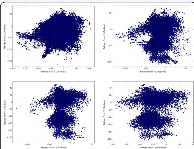
Figure 4: Progressive application of quality filtering thresholds to the filter training dataset. Plots show Y (EW) error vs. X (EW) error in microradians ( $\mu\text{rad}$ ). UL: SZA<75°; UR: AMU<2.52  $\mu\text{rad}$ ; LL: CSR>250 (25%); LR: Addition of 9\*MAD extreme outlier rejection. The bimodal N/S behavior is an artifact of a GLM focal plane anomaly and is addressed via hemispheric stratification of results.
