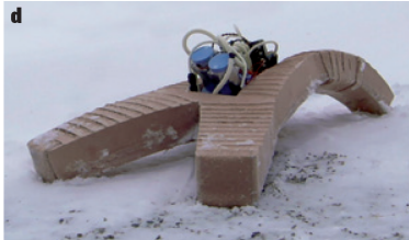
Figure 2: An existing soft robot showing crawling similar to what is proposed [35].
