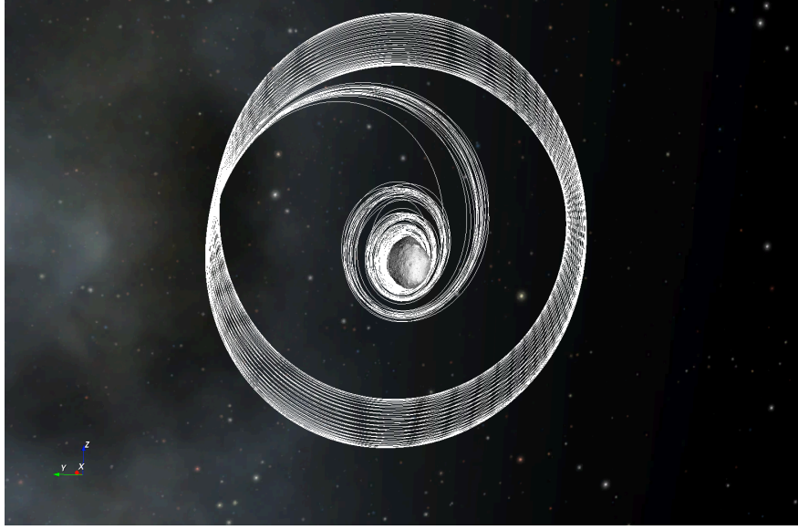
Figure 21: Monte-Carlo results featuring 20 AoES trajectory @ Itokawa, landing from a terminator orbit, with error added to the initial attitude, position and velocity components. The control law was reducing the semi-major axis only
