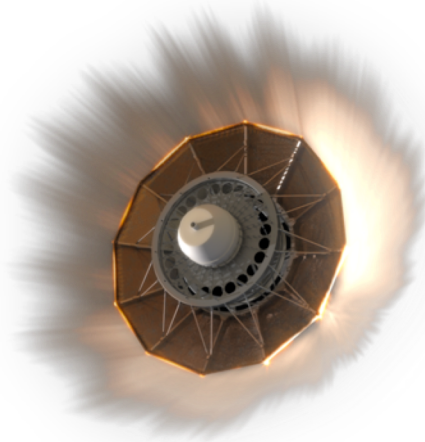
6 m diameter ADEPT-Venus in cruise (left) and entry (right) configurations
