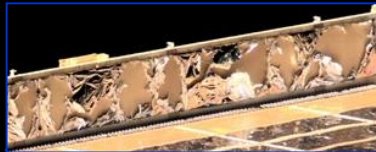
AO undercutting erosion of the P6 Port Solar Array Al-Kapton blanket box cover (1 yr)
