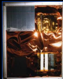
AO erosion of Kapton blanket
