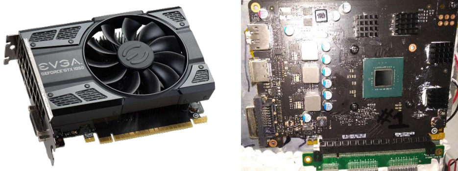
Figure 1: Nvidia GTX 1050 GPU with Heatsink (left) and As-Tested (right)
