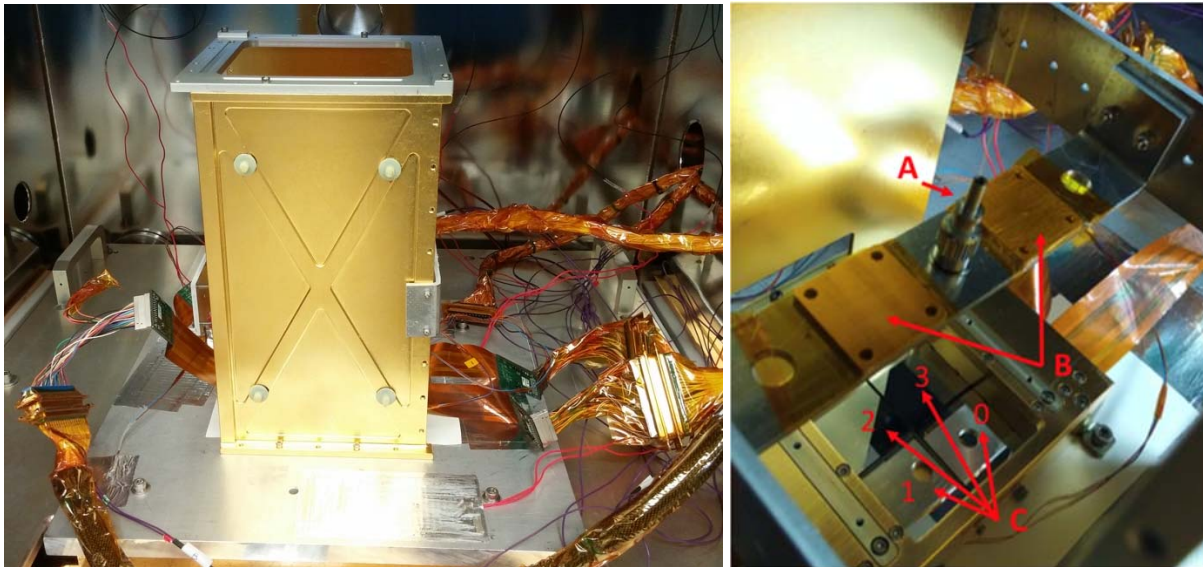
Fig. 4. Right: Tower that supports the Laser and X-ray sources; flexprints from the CCDs come out of each side. Left: A) End of the laser positioned above the CCDs; B) ^{55}\text{Fe} sources; C) Four CCDs in the DAM with their numbering convention.
