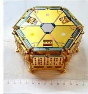
X-IFU scale calorimeter array mounted on testing setup with similar design as X-IFU Focal Plane Assembly
