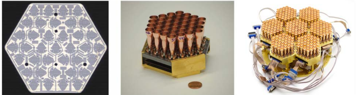
Fig. 3. Left: A 90-GHz 37-element array. Center: A complete 90-GHz sub-array prototype module. Right: Focal plane of the Cosmology Large Angular Scale Surveyor tiled with 7 sub-array modules.
