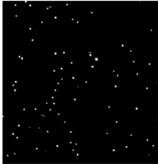
Fig. 2a. White areas show where light is visible above the noise floor on the flight CCDs pre-environmental testing.
