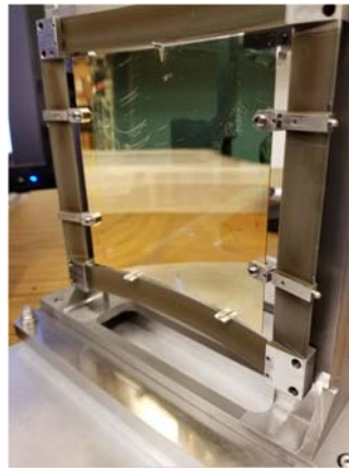
Fig. 4. Fit-check of test conical segment in new mount.
