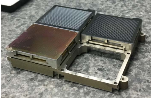
Fig. 4. Arcus flight-like grating window for four gratings. On the left is a flight-like CAT grating facet (grating membrane bonded to flexure frame). In the back are two facet dummies. (Image credit: E. Hertz, SAO).
