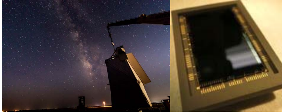
Fig. 6. Left: FIREBall undergoing on-sky calibration in Ft. Sumner, NM. Right: FIREBall detector with three-layer dielectric delivering QE > 60%.
