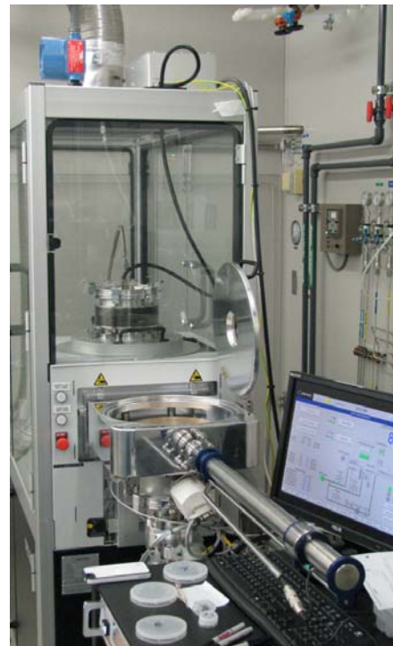
Fig. 1. Left and Middle: Band diagram of delta-doped and superlattice-doped silicon surfaces. Right: Superlattice doping is a molecular beam epitaxy (MBE) process performed in the 8"-wafer-capacity silicon MBE at JPL ®
