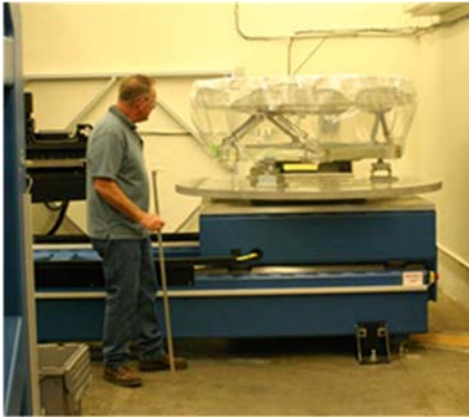
Fig. 1. 1.5-m AMTD-2 mirror being X-Ray CT scanned.
