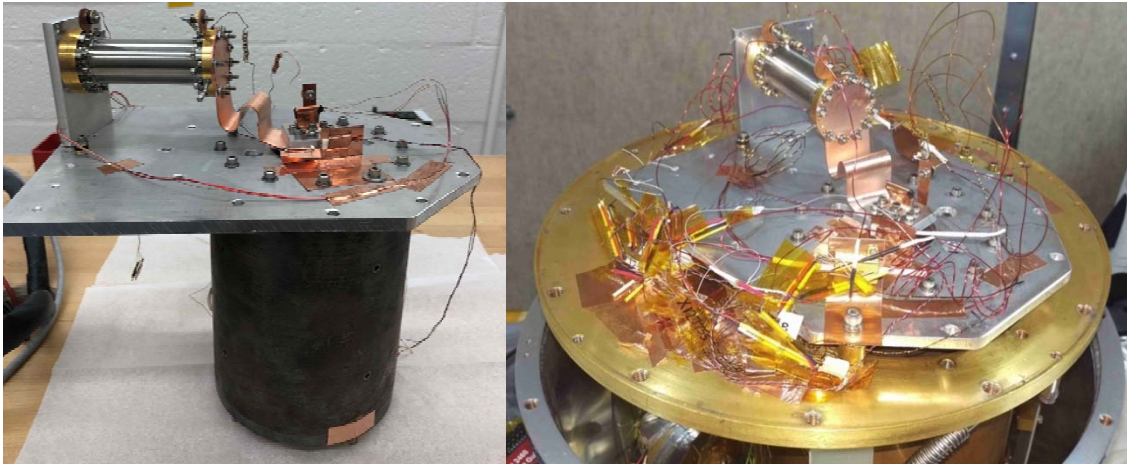
Fig. 4. Left: The single-stage 10-to-4-K ADR. Right: The ADR installed in a cryostat for testing.
