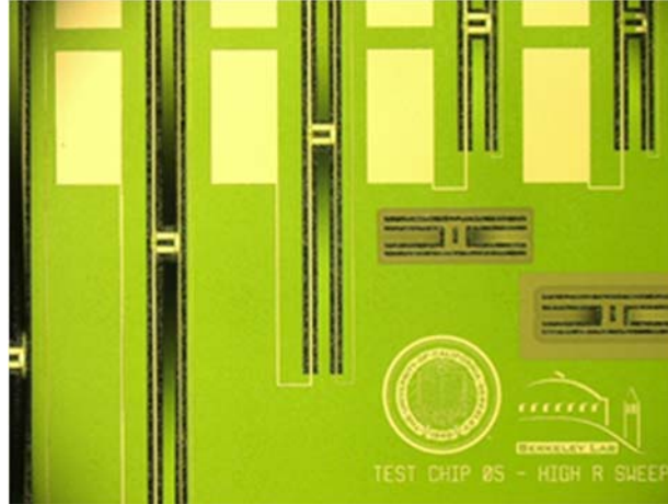
Fig. 4. Photograph of a LiteBIRD test chip fabricated at UC Berkeley with fabrication support from NIST for the ALMn TES. Results from initial test show that these bolometers are with a 10% of the T_c target and a factor of 2 of the normal resistance targets.
