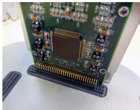
Fig. 11. External side of detector showing 80-contact feed-throughs ( \times 2 ) sealed with epoxy and a 64-channel preamp board plugged into one axis.
