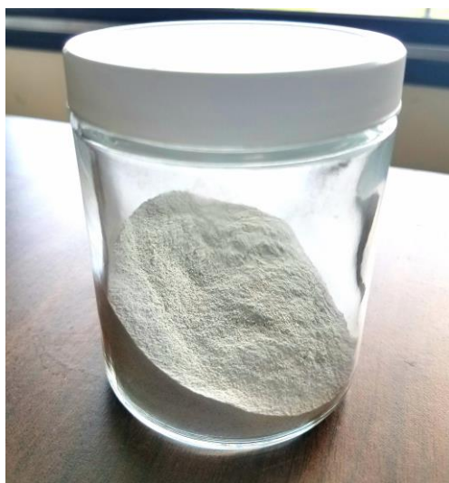
Figure 2. The experimental agglutinate-bearing, OB-1 base lunar highlands-type simulant.
