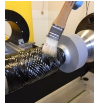
Top Right: Uni-directional tape placed over adhesive.
