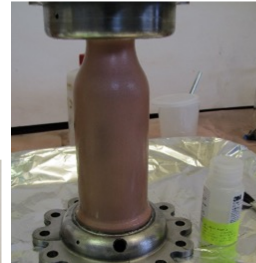
Surface prep of copper chamber (grit blast and AC-130-2 surface pre-treatment).
