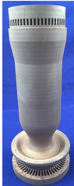
Additive Manufactured GRCop-84 Liners
