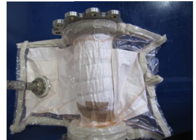
Vacuum bag setup prior to cure.
