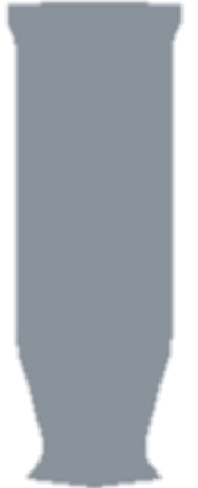
Template for ply 1 (Separate templates for adhesive and each ply accounting for thickness of material).
