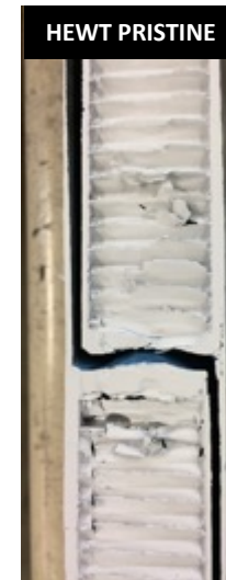
Failed HT Coupon
