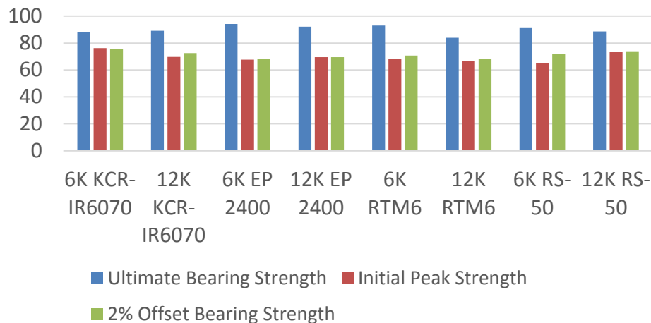
Single Shear Bearing- RTA Tests
