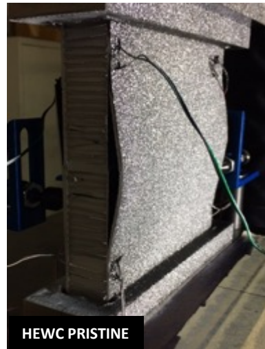
Failed HEWC Coupon
