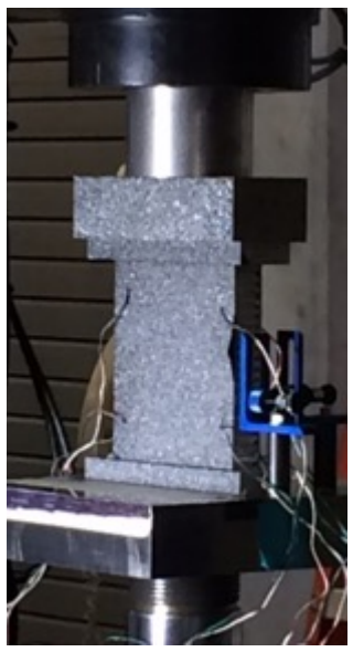
Test Setup of AEWC & HEWC Coupons
