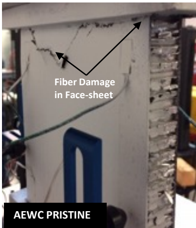
Failed AEWc Coupon
