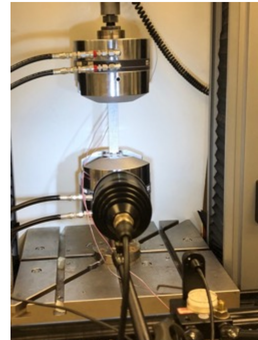
Photo of mechanical testing 3D woven coupon at GSFC.
