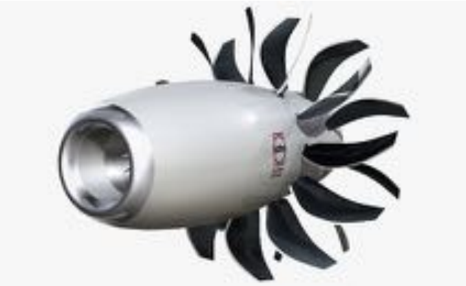
Modern contra-rotating open rotor engine design from CFM (12x10)
