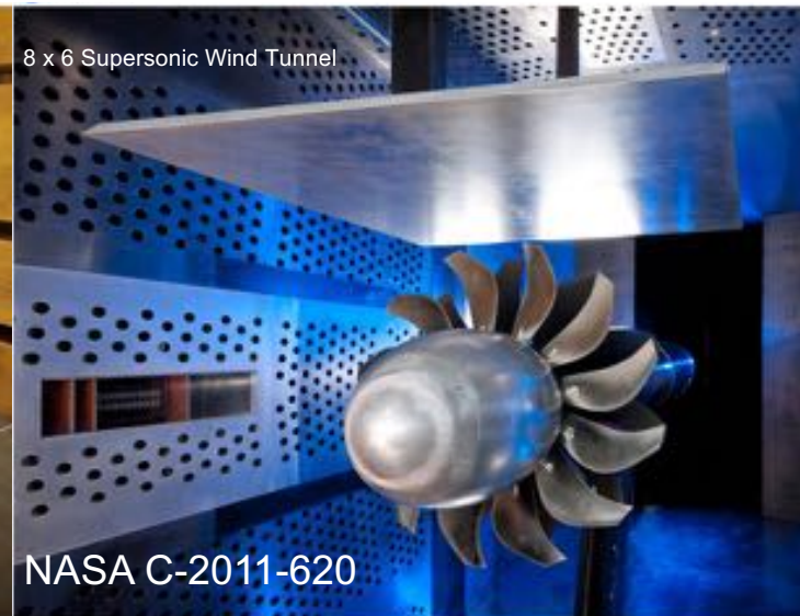
Modern contra-rotating open rotor engine design from CFM (12x10)
