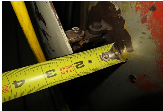
Figure 12 Vortex Generators Attachment Hardware
