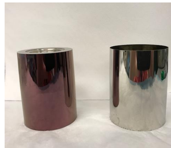
Mandrel ( left ) and replicated NiCo optic ( right )
