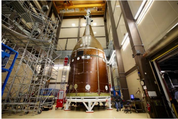
Figure 20: Orion Structural Test Article
