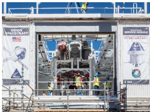
Figure 19: Orion Propulsion System Qualification Test Article
