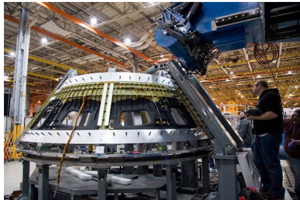
Figure 17: EM-2 CM Primary Structure Welding
