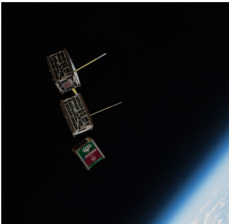
Figure 5. The Nodes spacecraft shortly after deployment from the International Space Station on May 16, 2016. The two spacecraft demonstrated new network capabilities critical to the operation of swarms of spacecraft. Image credit: NASA
