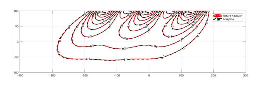
Steady state temperature profiles of PuMA and analytical solutions [5]
