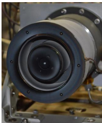
Figure 7: MaSMI Hall thruster
