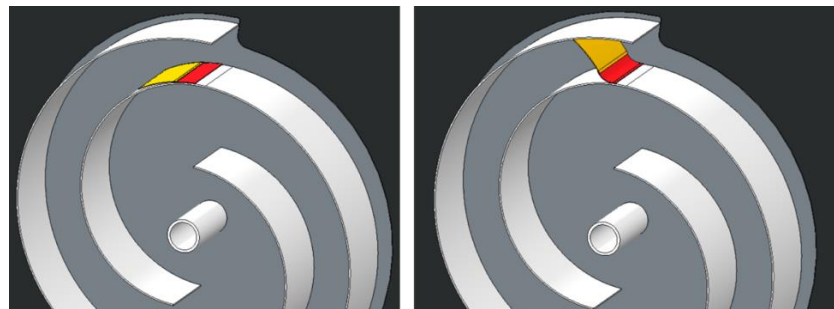
Figure 6. Bimetallic hinged door concept open (left) and sealed (right).
