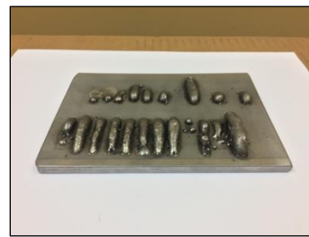
Figure 4. Set of AM tests using the 28 wt.% Si FeSi wire. The beads are solid, and minor cracks are observed on surface.
