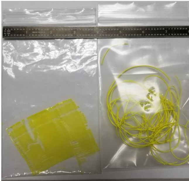
Figure 1. (Left) Showing PIM-1 mat coupon designed and printed by Georgia Tech, and (Right) raw PIM-1 fibers fabricated by chemically dissolving raw PIM-1 material and drawing it out as a continuous fiber. Figure 2. Showing heated CO 2 gas flow test cell setup where the CO 2 gas flowed across
