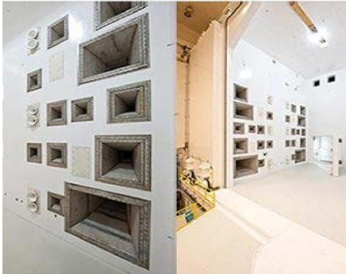
Figure 10: Reverberant Acoustic Test Facility horn wall is shown at left, and the overall chamber is shown at right.
