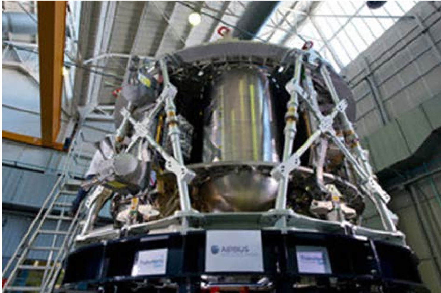
Figure 3: Orion European Service Module test article.
