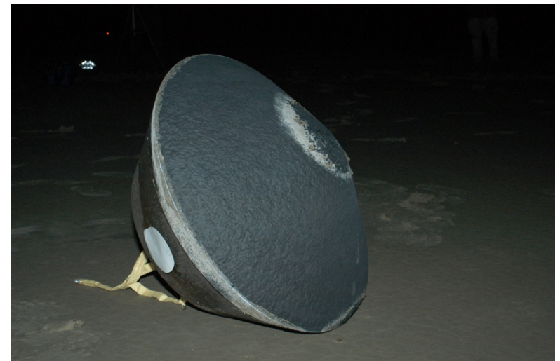
Stardust single piece, seamless heatshield
