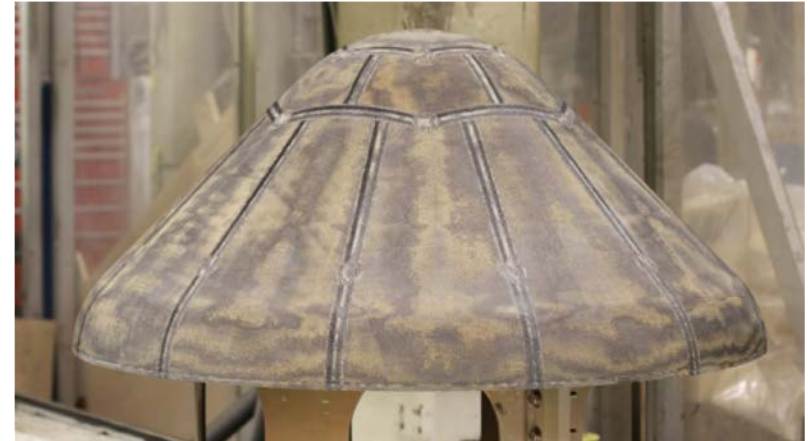
HEEET 1m Engineering Test Unit (ETU)
