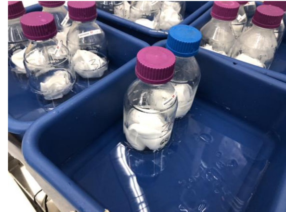
Quenching shocked samples in ice bath
