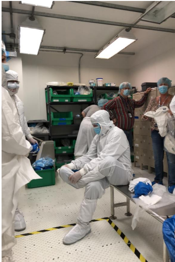
Booties, hairnet and mask followed by hood, bunny, suit, boots, gloves and wrist tape.
