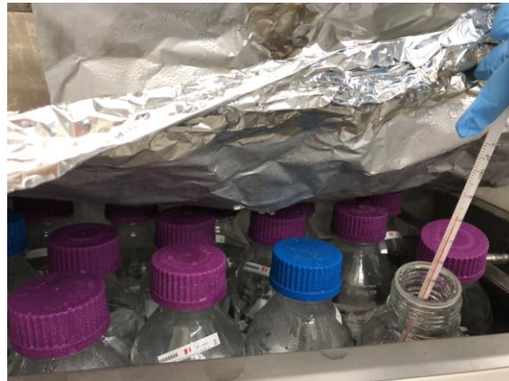
Heat shock of the extracted samples at 80°C for 15 minutes
