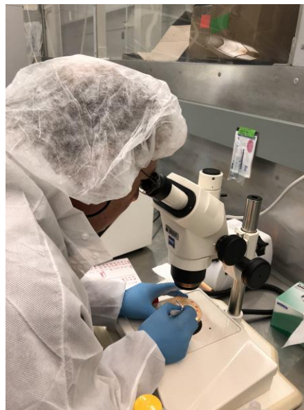
Visual enumeration of colony forming units after incubation at 32°C for 24, 48, and 72 hours
