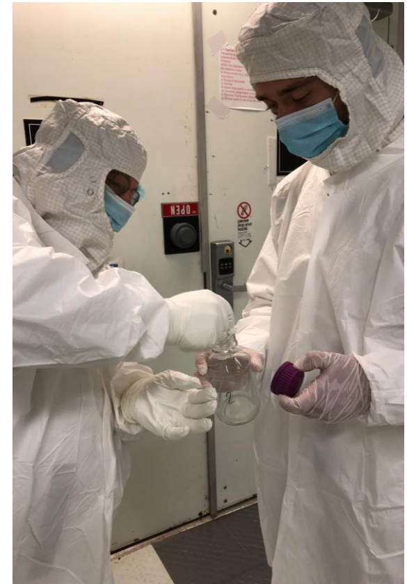
Polyester wipe inserted into sterile glass bottle with deionized water for extraction.
