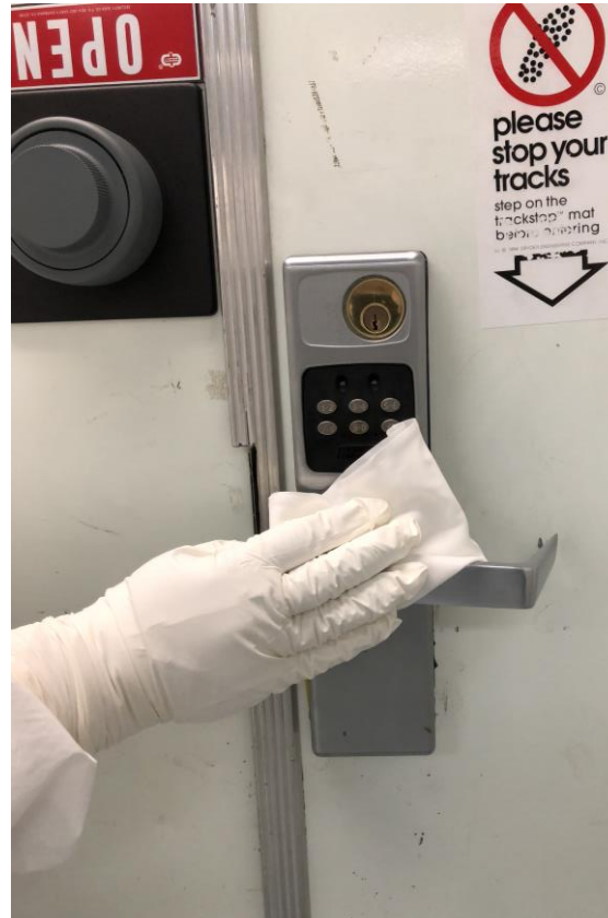
Spacecraft hardware and transfer surfaces are sampled by wiping or swabbing.
