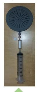
Use syringe to inject ~50mL water into production pack. Trash microbial filter.
