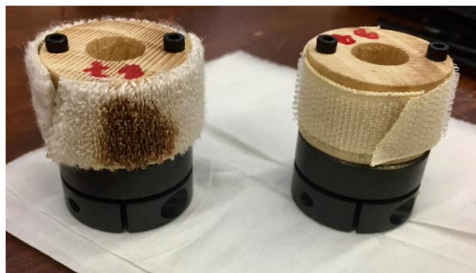
Figure 11.—Stained sample of International Space Station (ISS) hook-and-loop tape prepared by cut-and-wash method to extract embedded ISS debris particles for transmission electron microscopy (TEM) and scanning transmission electron microscopy (STEM).
