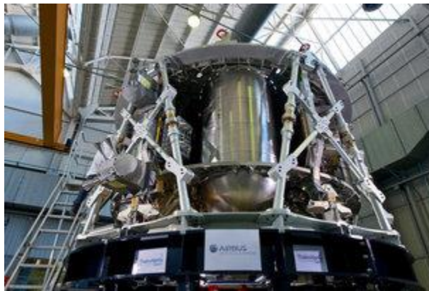
Figure 3: Orion European Service Module (ESM) test article.
