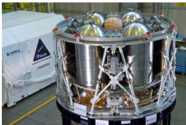
Figure 5: European Service Module (ESM) test article.
