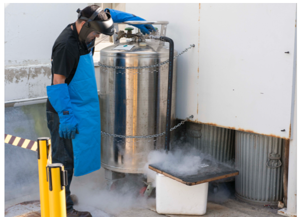
Figure 11: Collector/Target immersion in \text{LN}_2 bath for super cooling.
