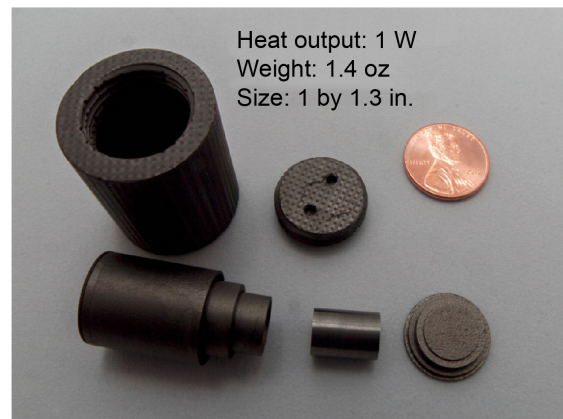
Figure 11.—Radioisotope heater unit components (Ref. 28). (a) Radioisotope heater cutaway view. FWPF is a carbon-carbon composite woven with perpendicularly oriented graphite fiber and PG is pyrolytic graphite. (b) Radioisotope heater unit and components and size comparison. Heat output of 1 W, weight of 1.4 oz., dimensions of 1 by 1.3 in.
