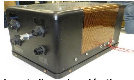
Zener-diode controller packaged for thermal vacuum.
