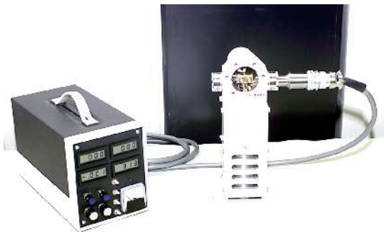
Portable K-Band Cryogenically Cooled Low-Noise Receiver for the Direct Data Distribution Experiment
