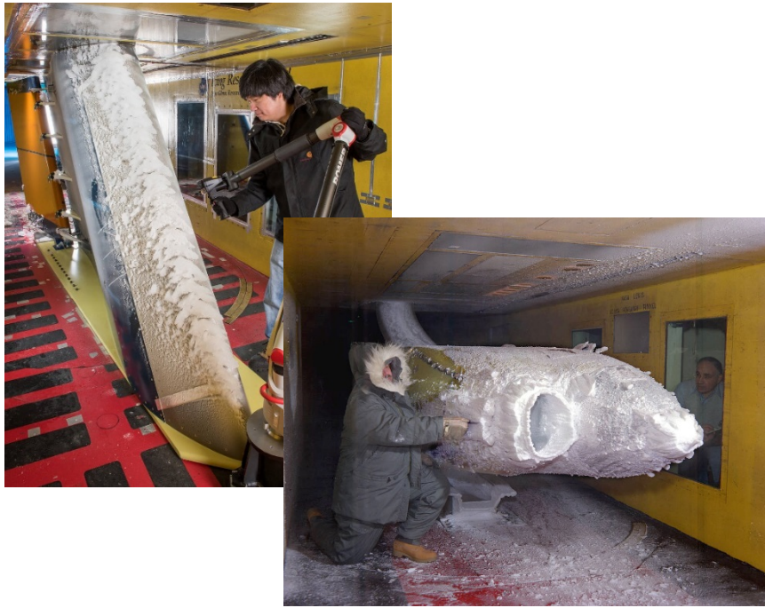
Ice Accretion Testing – Icing Research Tunnel
