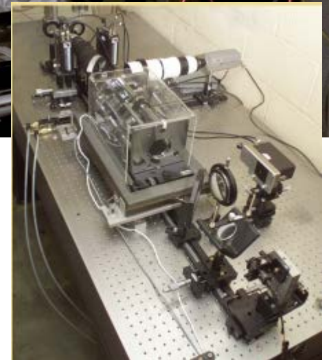
Typical Setup for Analysis and Detection of Rayleigh Signals
