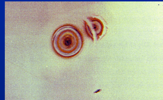
Penetrations, and commonly associated ringed structure, in silver-Teflon thermal blanket
