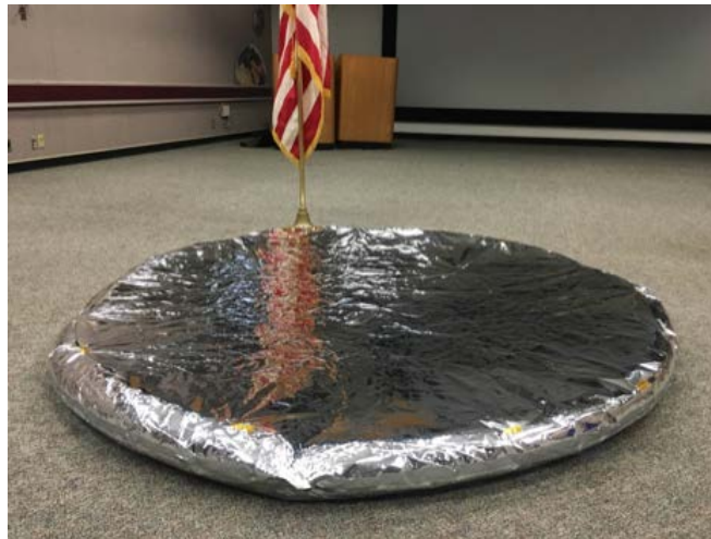
Figure 3.15. Deployable Mylar sheet with inflatable Mylar and vinyl torus; 2-meter diameter.
