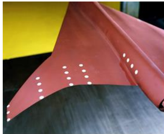
Figure 16. Targets on a model used for VMD measurements.
