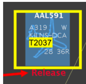
Figure 4.15. Alert to Release From Hardstand.
