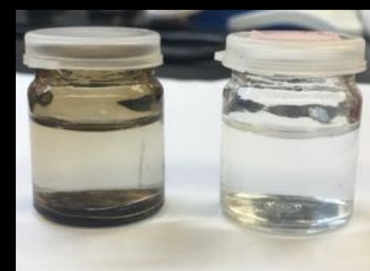
Comparative image of an irradiated vessel (left) and a control vessel (right). Concerns of shielding led way to a materials consideration across a variety of different vessel types, as shown in the table.
