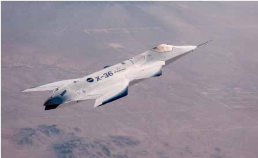
The X-36 was a remotely piloted, subscale, tailless aircraft technology demonstrator. NASA
