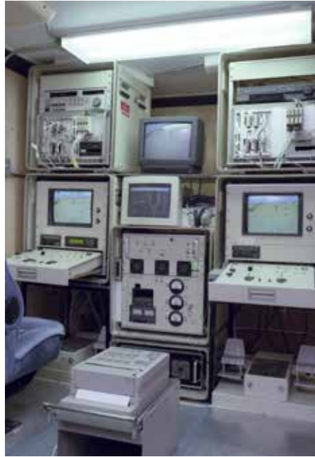
The Perseus ground control station contained simple joystick and switch controls, ground-track/location monitor, head-up display, and flight instruments displayed on CRT screens. NASA
