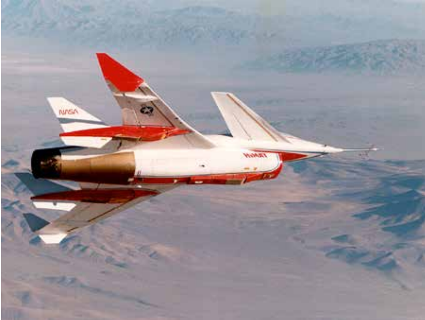
The HiMAT vehicle was a subscale representation of a notional future fighter design incorporating such features as canards, winglets, and supercritical wings. NASA
