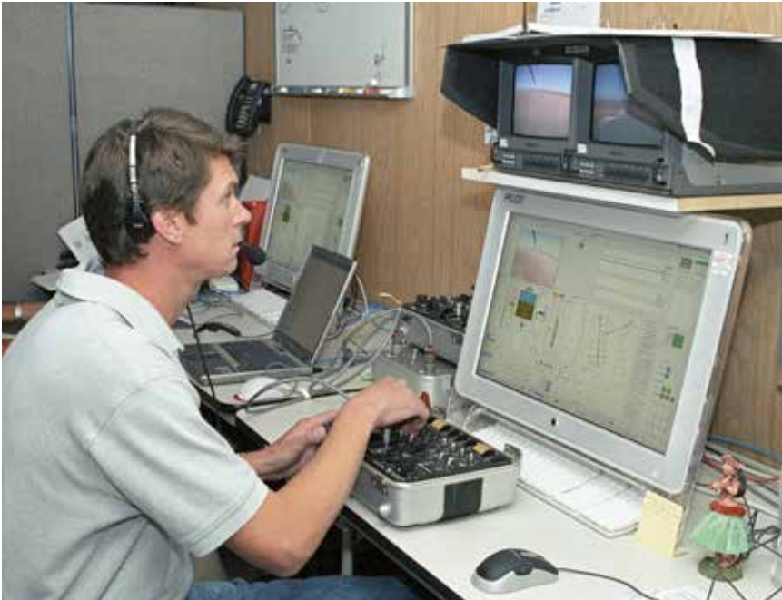
AeroVironment developed a pilot's station similar to those typically used to fly remote-controlled models. Here, pilot Wyatt Sadler uses the "flight station in a box" to fly the Pathfinder. NASA
