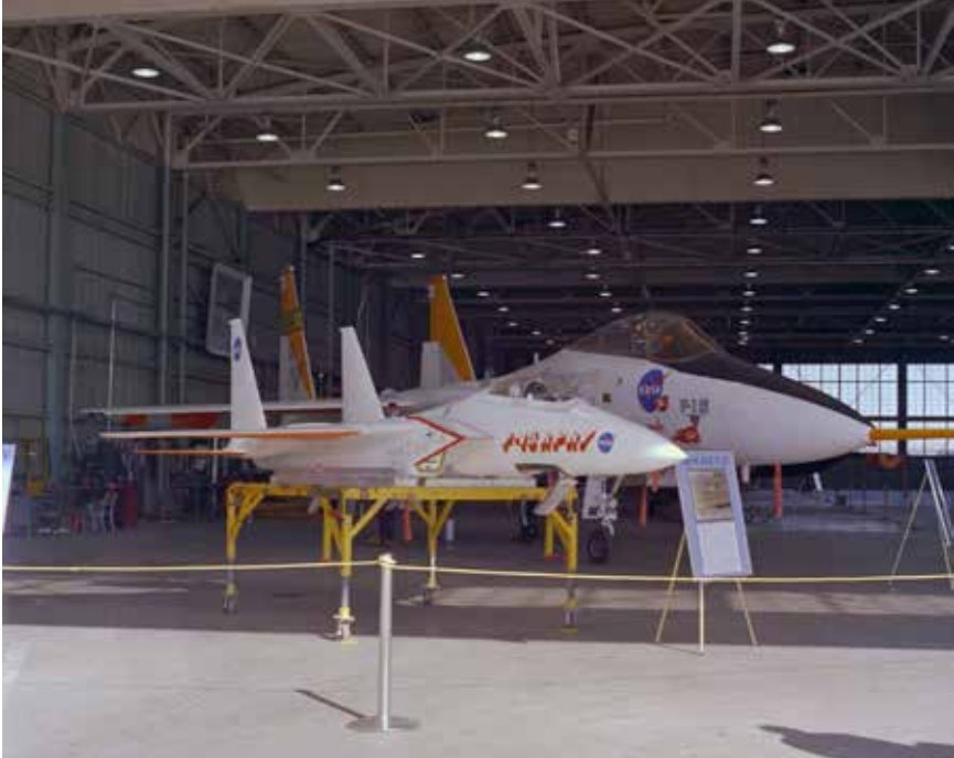
Use of a three-eighths-scale remotely piloted model of the F-15, seen here beside its full-size counterpart, allowed researchers to conduct hazardous tests without risking the pilot's life. NASA
