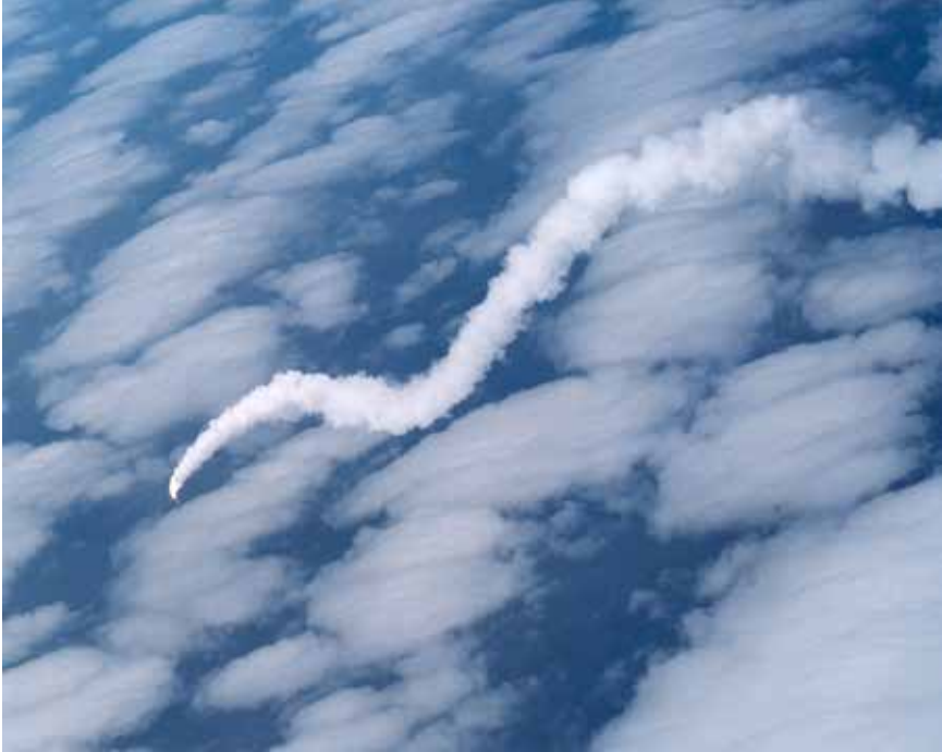
Divergent roll oscillatory motion caused by excessive control-system gain resulted from inadequate analytical modeling that allowed engineers to overestimate system safety margins. NASA
