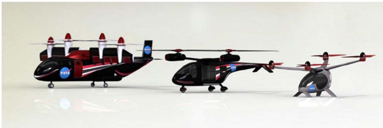
NASA reference models. Left to right: NASA reference model 3 (14 passenger TiltWing), NASA reference model 2 (six passenger side-by-side), NASA reference 1 (personal quadrotor).
