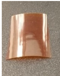
20x25 mm Kapton film, typical of that used for the deposition substrate
