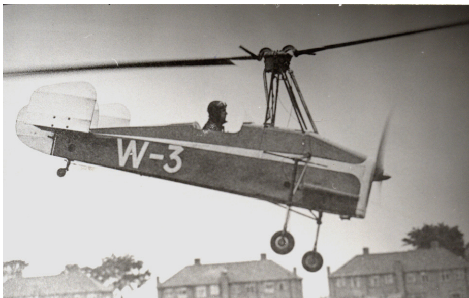
Figure 19: The Weir W-3 executing jump-takeoff at Hanworth Aerodrome.
