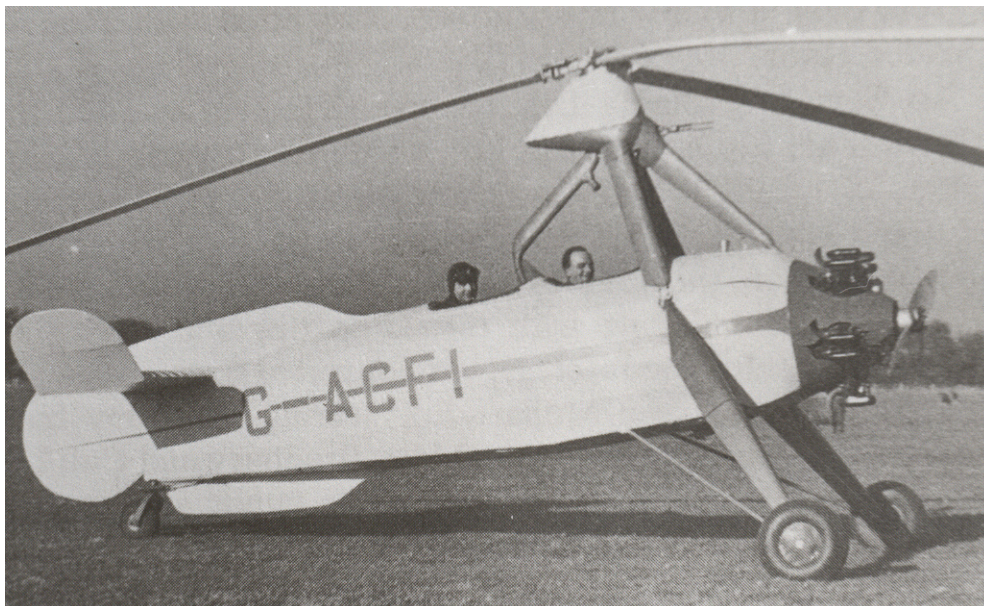
Figure 6: The C.30 Autogiro G-ACFI with standard fixed-pitch rotor before tests with autodynamic hub.
