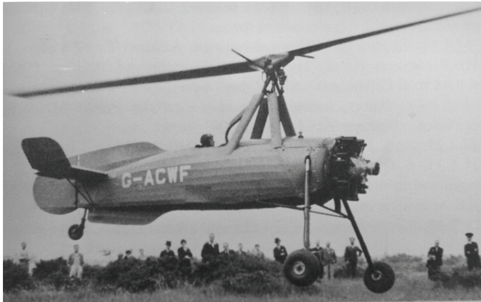
Figure 18: The C.30 Mk.III executing jump-takeoff at Hounslow Heath, 17 July 1936.
