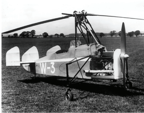
Figure 12: The Weir W-3 with engine cowl removed.
