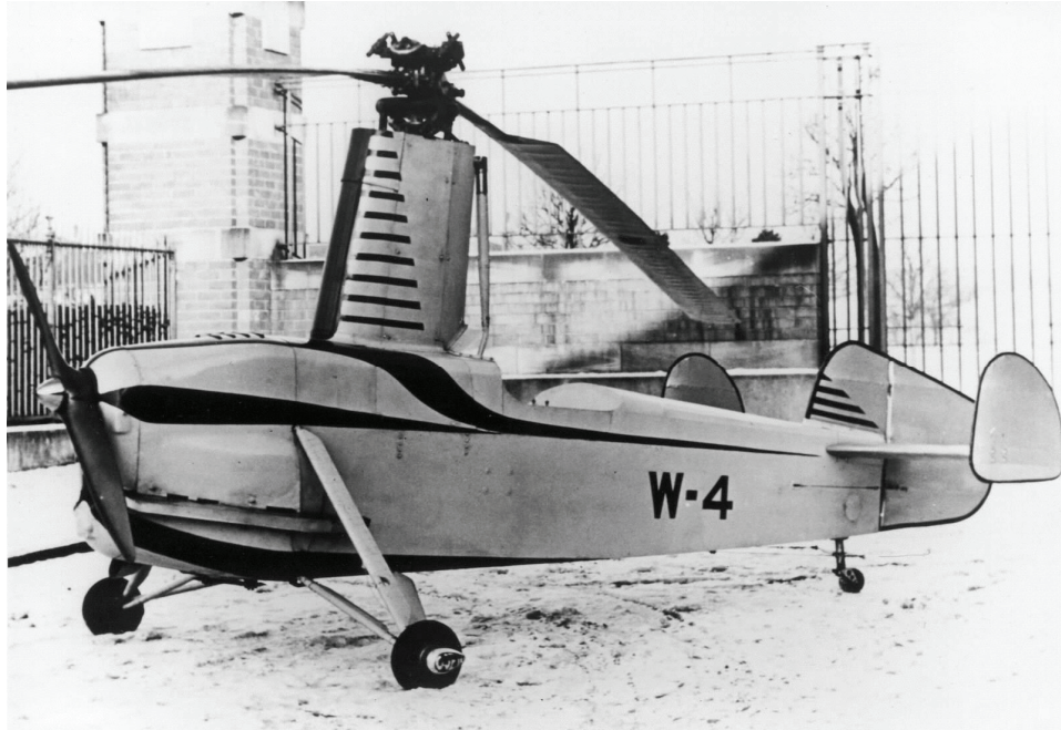
Figure 22: The Weir W-4 with adjustable direct-takeoff rotor hub (photo courtesy of the Weir Group).
