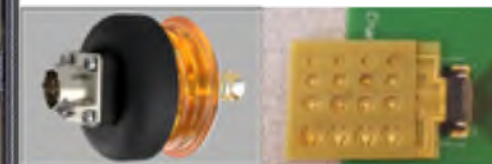
Printable Electronics: LSS Pressure Switch (Left); UV Radiation Sensor (Right)
