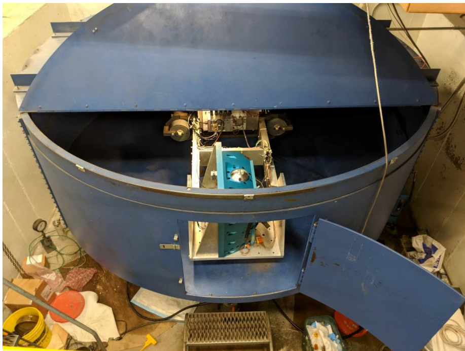
Figure 9.—110-W e Stirling Radioisotope Generator Engineering Unit Stirling Convertor Assembly 2 installed in centrifuge ready for axial static acceleration exposure.
