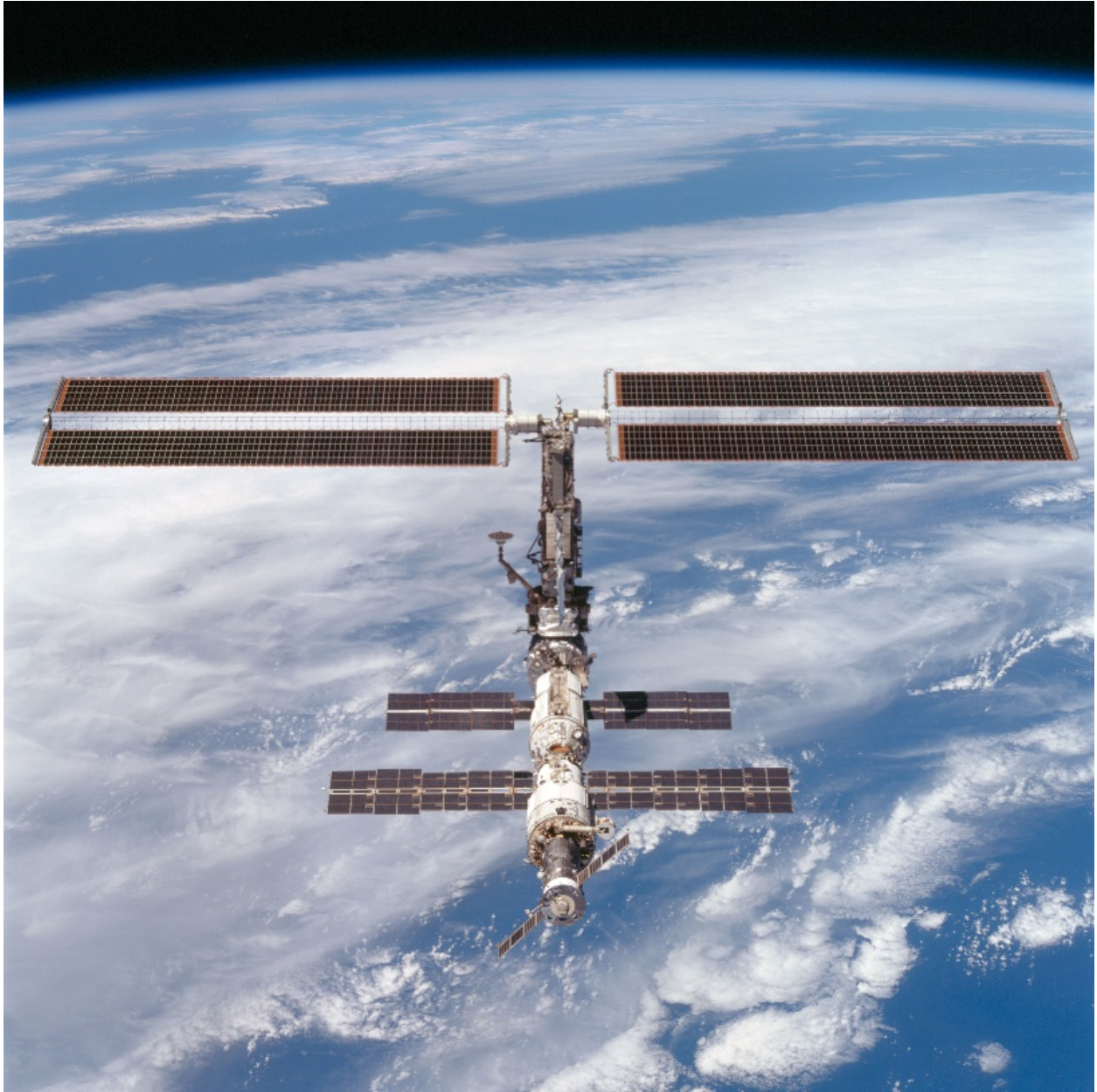
Figure 56.—International Space Station configuration in December 2000. From bottom to top: Soyuz, Zvezda Service Module, Zarya (Functional Cargo Block), Node 1 (Unity), P6 (sts097-704-074).
