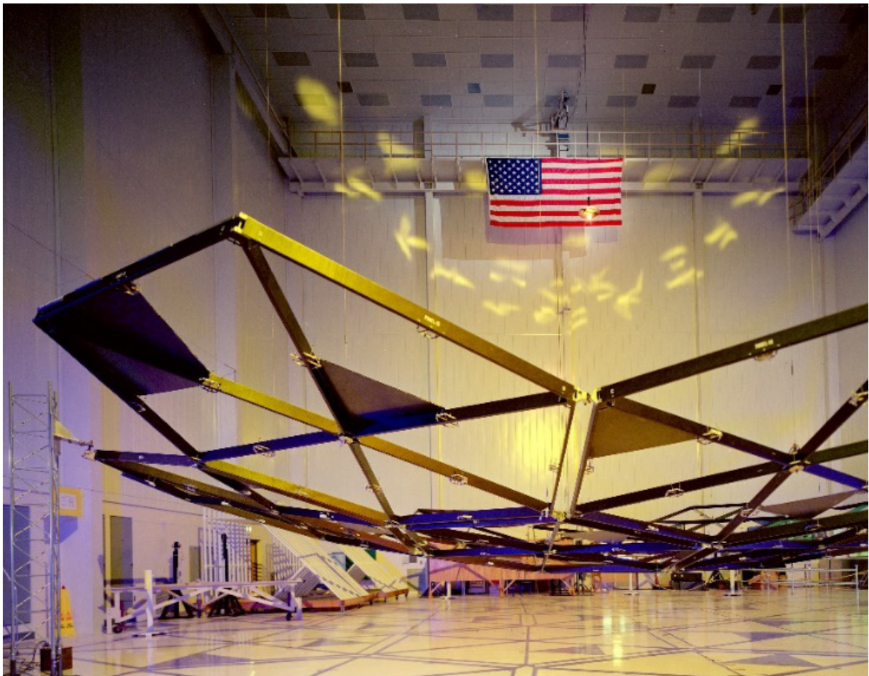
Figure 41.—SD Concentrator optical testing in PSF (C-1990-8258).
