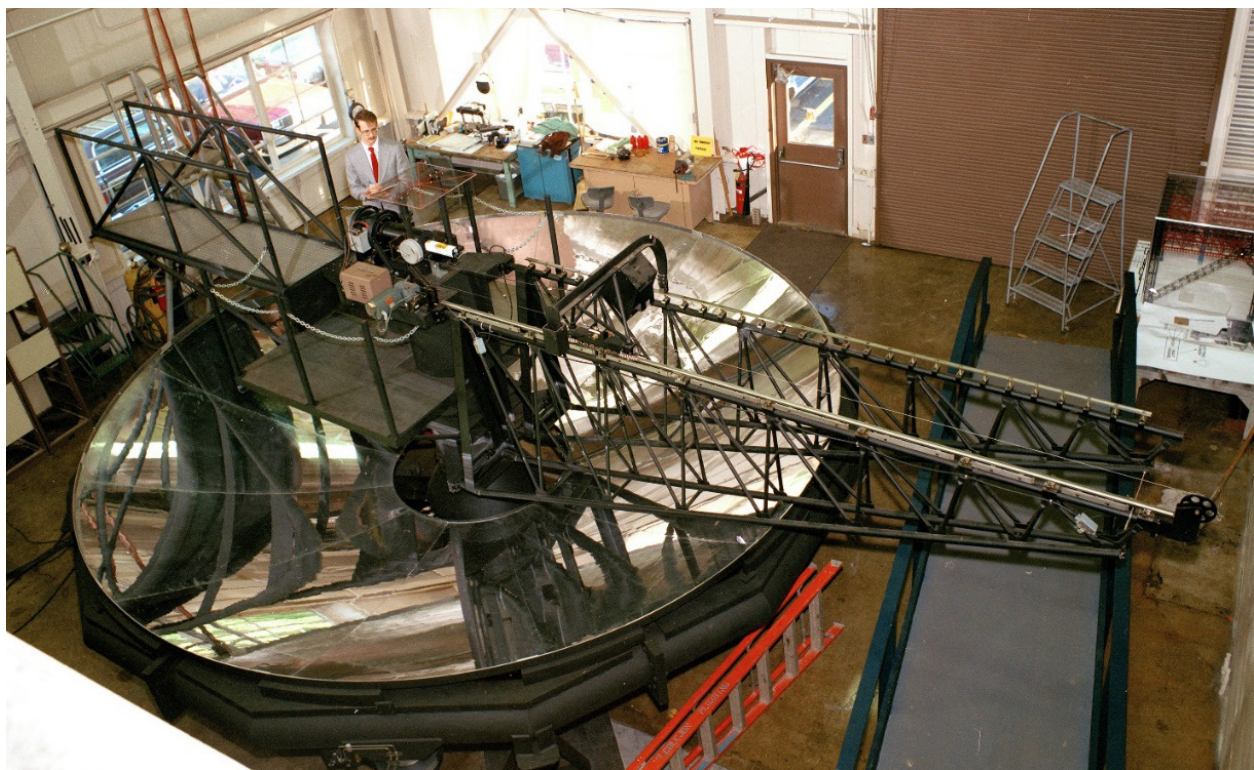
Figure 25.—Michael Ciancone, lead engineer for the concentrator testing, inspecting a development unit in the solar concentrator optical test facility at Lewis (C-86-7828).
