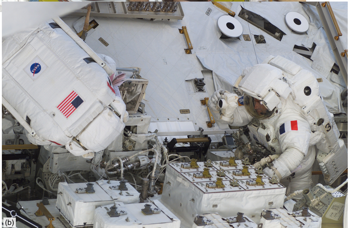
Figure 108.—(a) Astronaut Edward M. (Mike) Fincke, Expedition 9 NASA ISS science officer and flight engineer, holding a spare Remote Power Controller Module (RPCM), and then (b) during an EVA to replace a failed RPCM with the spare (iss009e10554 and S111E5183).
