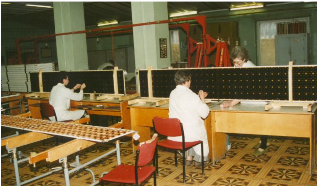
Figure 46.—Hand-sewing U.S. blankets into Russian frame for Mir Cooperative Solar Array. Photo taken in Russia.
