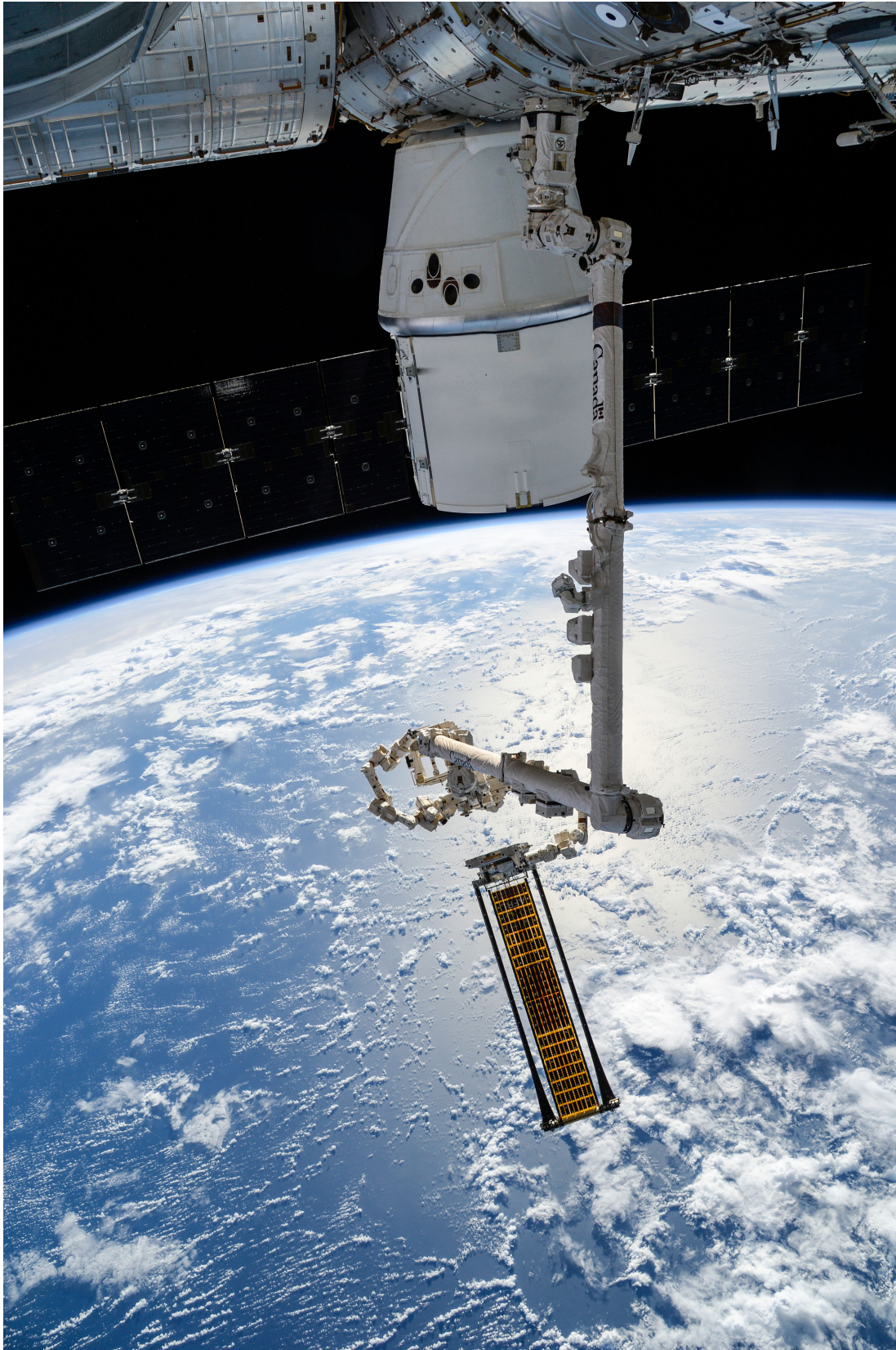
Figure 104.—The Roll-Out Solar Array experiment attached to the SSRMS, with the Dragon vehicle in the background (iss052e086009).
