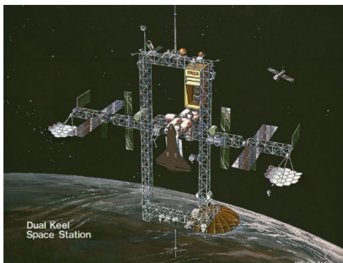
Figure 24.—Final phase B enhanced configuration with photovoltaic and solar dynamic power modules.
