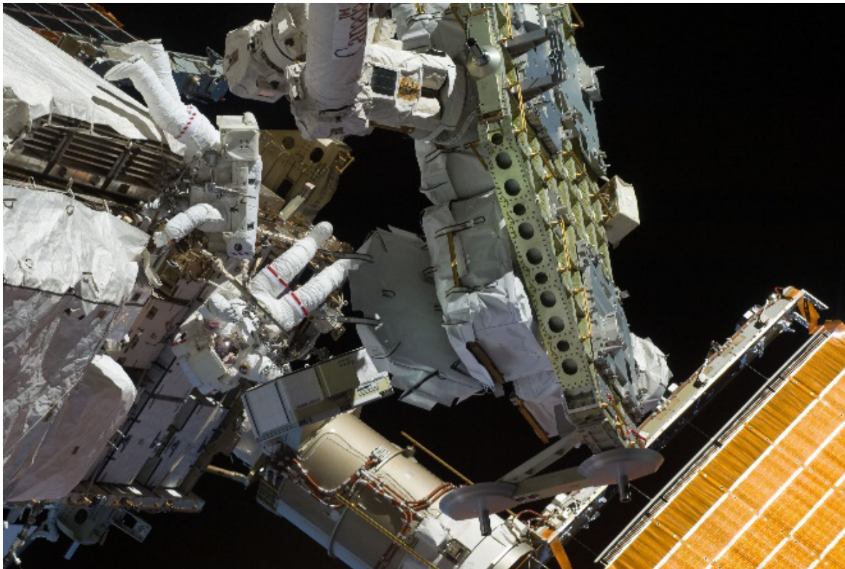
Figure 97.—Astronauts removing old 2B NiH 2 battery (S127E008440).
