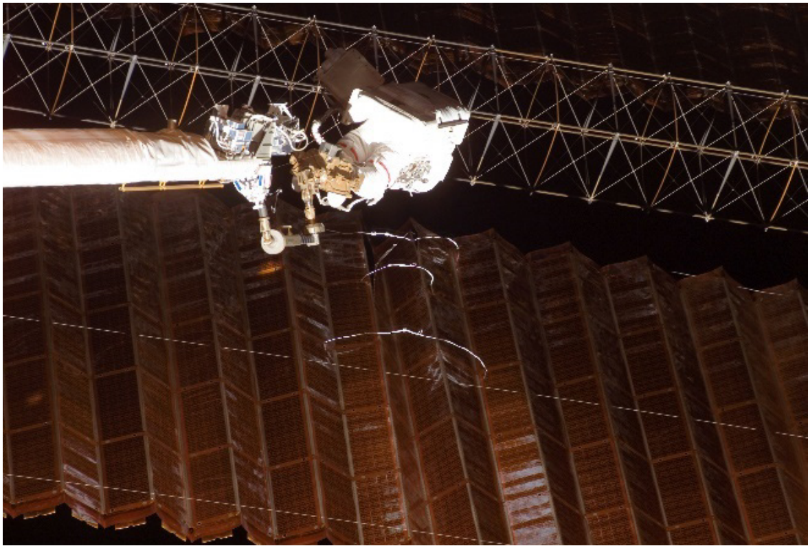
Figure 82.—Repaired 4B solar array (ISS016E009196).
