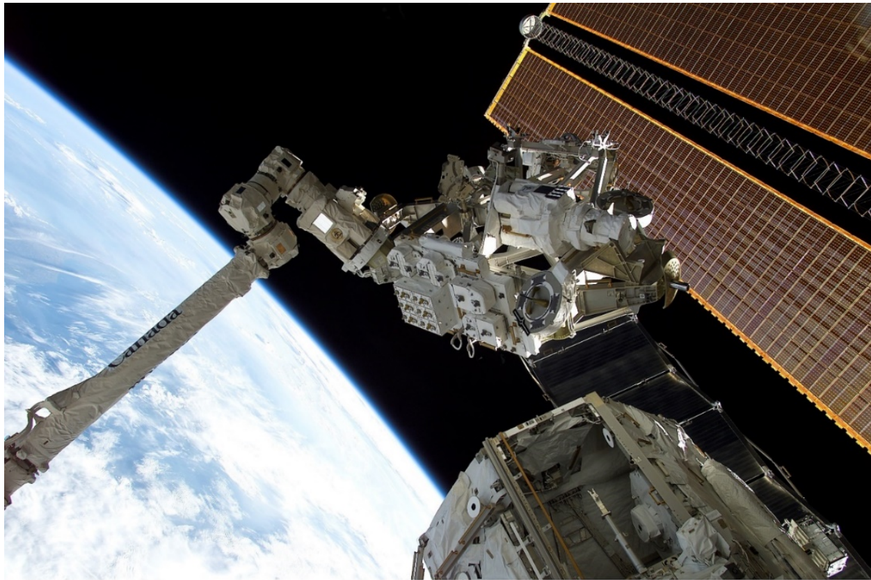
Figure 9.—Mobile Base System grappled to Canadarm2 Space Station Remote Manipulator System during STS-111 in June 2002.
