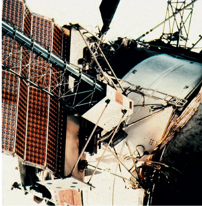
Figure 47.—Base of Mir Cooperative Solar Array mounted to Mir Kvant-1 module.
