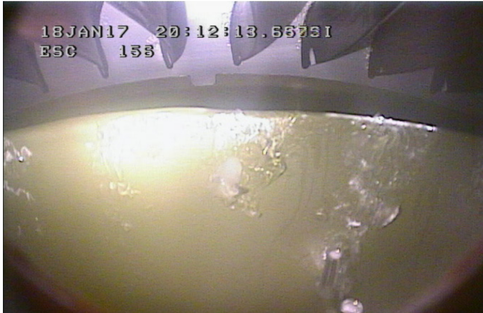
Figure 19.—For Escort 156, there was ice accretion on the shroud, without horns.
