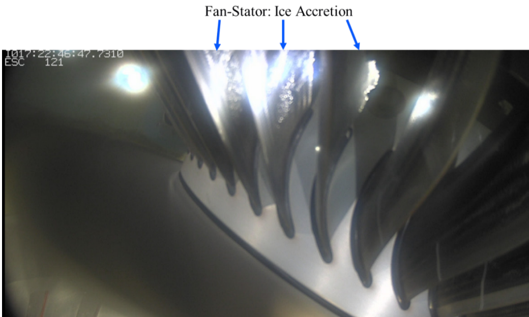
Figure 11.—Video camera view of the fan-stator showing that ice accretion occurred there during Escort data 121.
