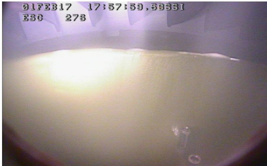
Figure 22.—Ice collection on the splitter-lip with rapid shedding, is not considered ice accretion since it does not grow (Escort 276).
